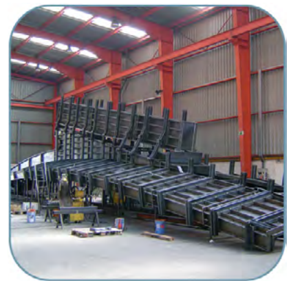
Formwork for a pier bridge in Morocco. 2009
