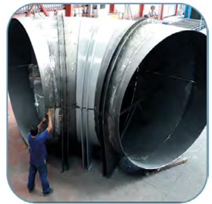
Elbow for dam drainage. 2020
