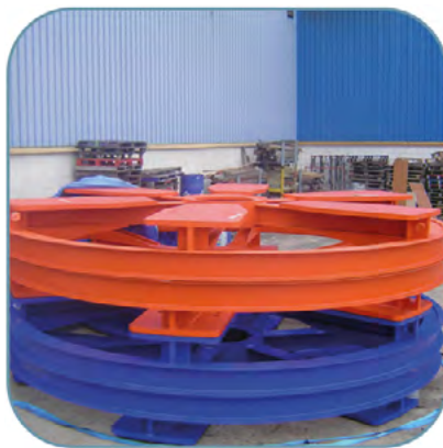
Reinforced plates for turning wind blades. 2010
